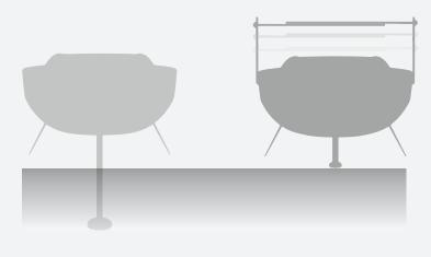
The operation to arrive in shallow water coves, ports and marinas was never so easy to be accomplished. By a push of a button, both sides (port and starboard) SBS wings will rotate up coming out from the water and stored above the deck.\*
