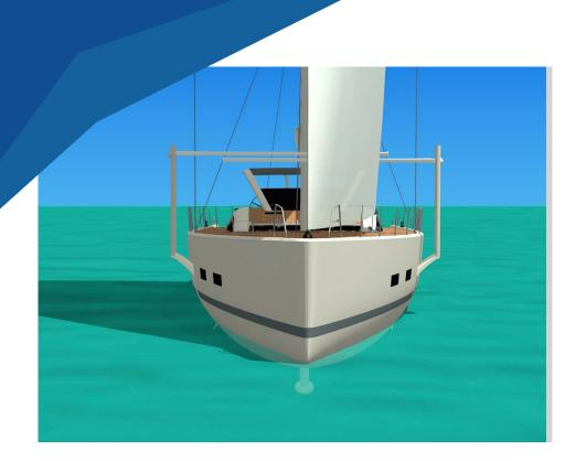
SBS wings are easy accessible for the crew above the deck , facilitating maintenance such as polishing and cleaning; or, if while sailing, plastic, trash or sea weed gets caught, it can easily be removed by placing up the wings. The wings also can be used for a smooth transfer of crew members while in open waters avoiding unnecessary swims in cold or unclean waters.
