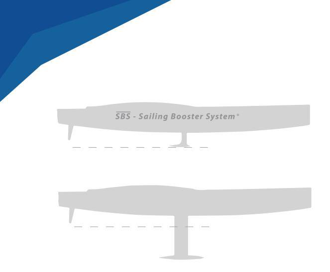
The lift wing may reduce bulb keel weight up to 68%.
