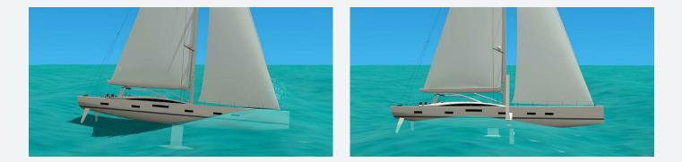
At high speeds, sailboats have a vast pitch acceleration on the bow, causing water to embark and the crew must keep distance from the bow in order to avoid accidents. The SBS system generates forward lift to the static center of buoyancy reducing while sailing the vessel's pitch and the quantity of water embarked due to the bow waves.
