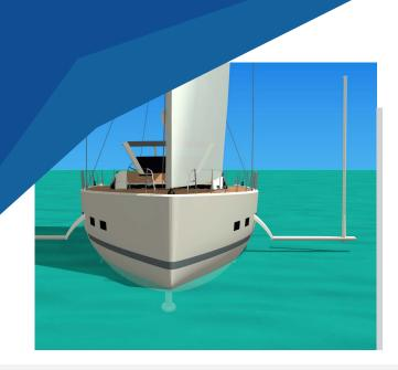
In aft and broad winds you will be able to remove both SBS wings from the water keeping them up or in horizontal position. Wet surfaces and drags will be kept to a minimum.
