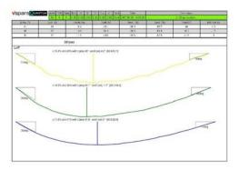
With this photo, we can turn this shape into numbers to describe the shape. Based on the numbers, depth, draft position, entry angle, and exit angle, we can advise on the level of performance the sail will provide. Often, we can adjust the luff or leech to help the sail perform longer.
