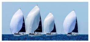
Downwind sails need to be viewed off the boat to see how they fly. The goal with asymmetrical spinnakers is to have a sail that flies like a symmetrical spinnaker downwind and sails like a genoa when reaching. A variety of shapes allow boats to sail off the wind from a 50-165 true wind angle.
