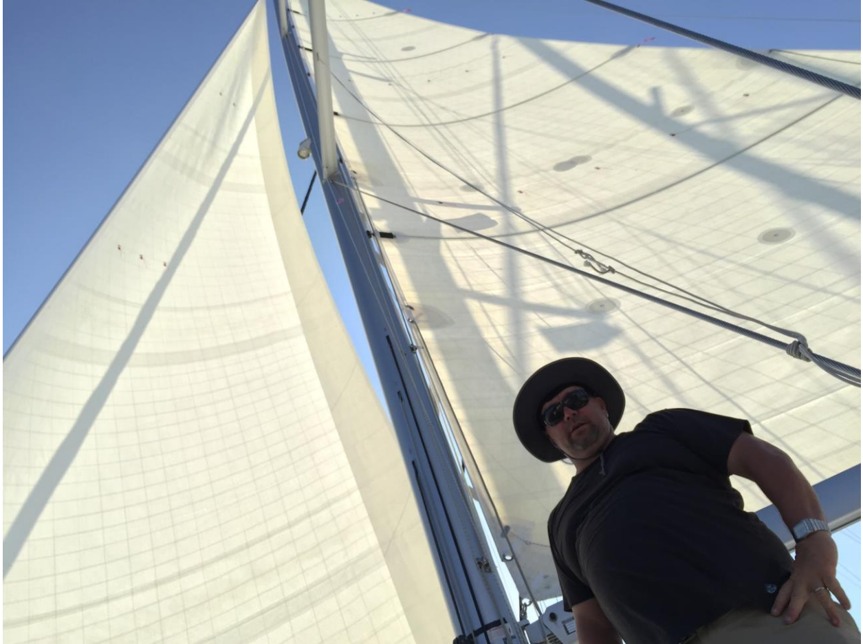
The composite structure is clearly visible on the test sails fitted and ready for sailing.
