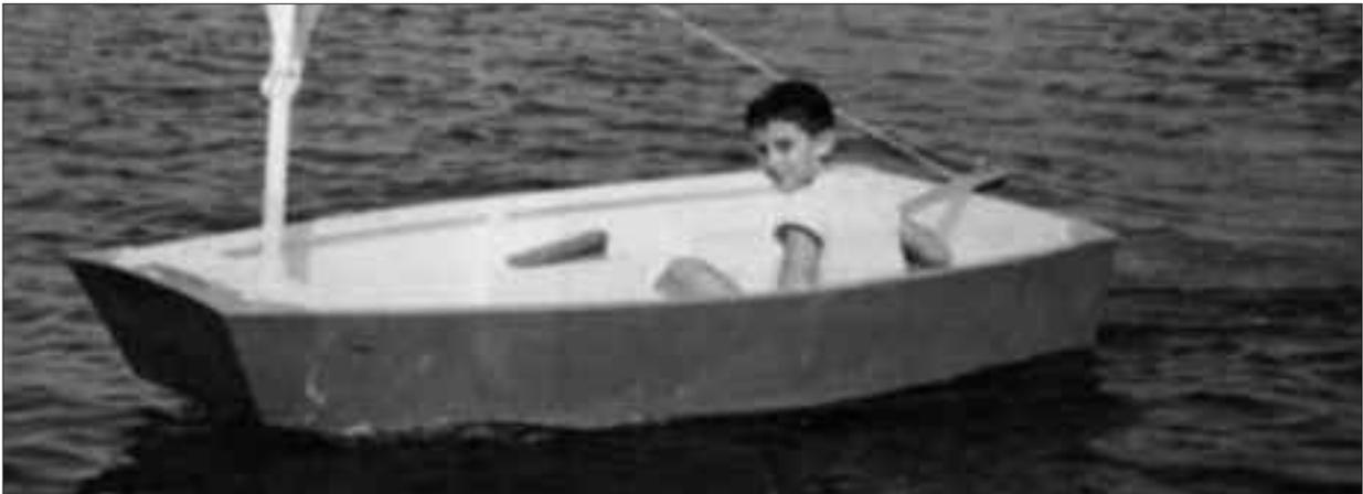
hulls. We boys took it from there, fastening the corner caps, installing the bow thwart and mast step, scraping off the glue that dripped down, sanding, painting, shaping the rudder and dagger board edges, bending the rudder fittings from galvanized sheet metal in the vice at the school woodworking shop, and tying the sail to the mast with venetian blind cord from the hardware store. Dickie Moore, a local sail maker, built the sails from common duck cloth. The mast was a 1 1/2" dowel from the
