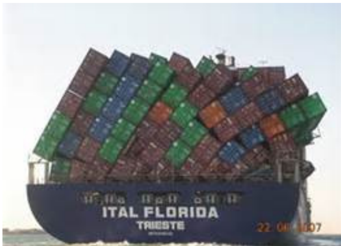
Bad weather caused this shipping container stack to topple
