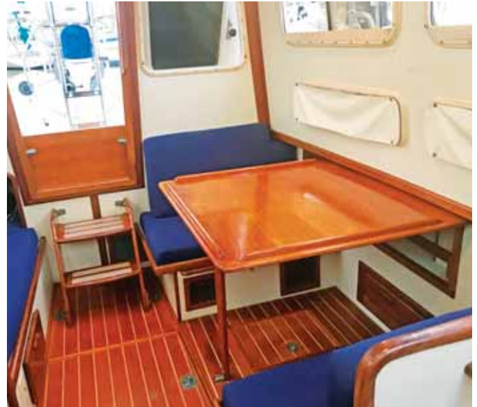
The port dinette has a large table that can drop down to form a bunk.
