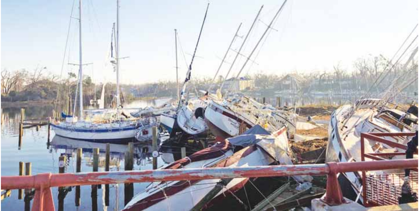
This is a photo of a safe harbor marina (hurricane hole) that saw quite a bit of damage due to tornadoes. The boats pictured were tied up together and the tornado spun the boats around and they ended up along the shore.
