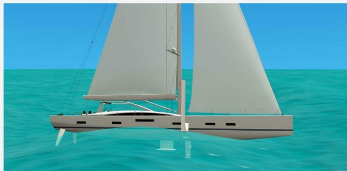
At high speeds, sailboats have a vast pitch acceleration on the bow, causing water to embark and the crew must keep distance from the bow in order to avoid accidents. The SBS system generates forward lift to the static center of buoyancy reducing while sailing the vessel's pitch and the quantity of water embarked due to the bow waves.
