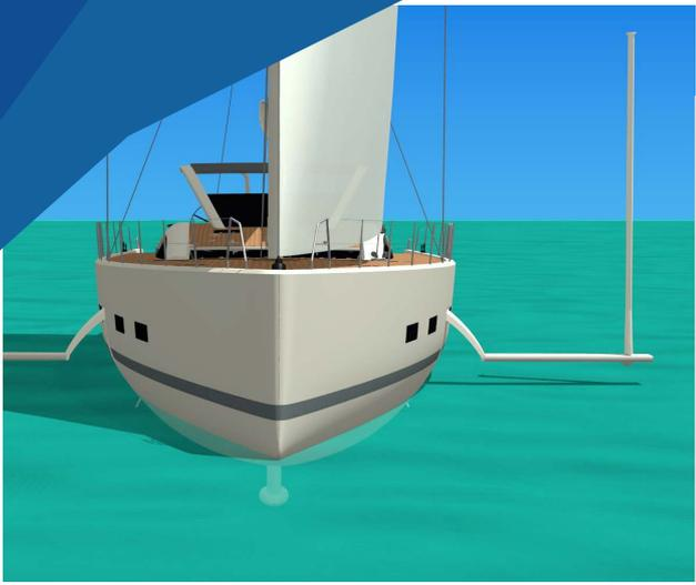
In aft and broad winds you will be able to remove both SBS wings from the water keeping them up or in horizontal position. Wet surfaces and drags will be kept to a minimum.
