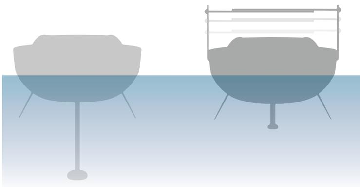
While the SBS wings are placed above the deck, on the upright position, the sailboat original beam is maintained. Less Marina draft for the any size of sailboat, is not a dream anymore . **It is the SBS reality.**
