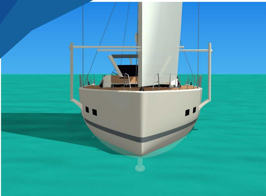
SBS wings are easy accessible for the crew above the deck , facilitating maintenance such as polishing and cleaning; or, if while sailing, plastic, trash or sea weed gets caught, it can easily be removed by placing up the wings. The wings also can be used for a smooth transfer of crew members while in open waters avoiding unnecessary swims in cold or unclean waters.
