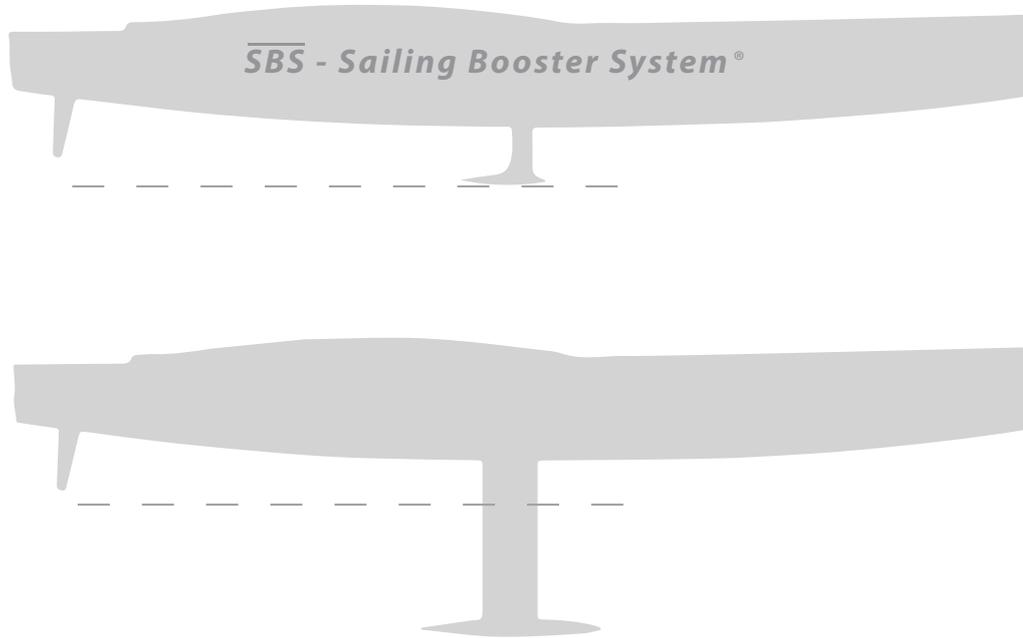
The lift wing may reduce bulb keel weight up to 68%.
