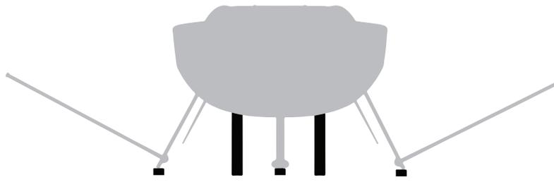
SBS wings can be stored in the upper right position or placed sideways in order to act as extra support on shore, increasing vessel's stability in high sideways wind.
