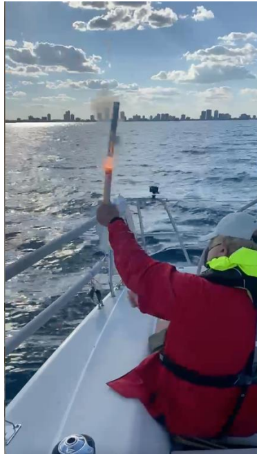
LAUNCHING A SOLAS ROCKET RED PARACHUTE FLARE NOTE THE ROCKET LEAVING THE TUBE.
