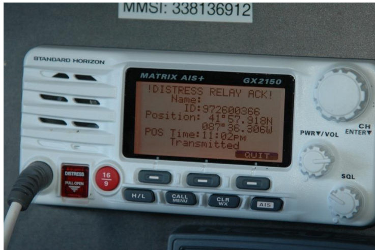
VHF RADIO SHOWING DSC MESSAGE FROM PERSONAL MOB DEVICE. NOTE, ONLY THE BOAT WITH ITS MMSI # PROGRAMMED INTO THE THE DEVICE WILL RECEIVE THIS MESSAGE.
